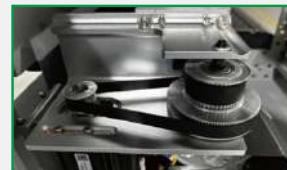
X, Y axis motion transmission structure upgraded to provide more stable movement to ensure printing quality.
