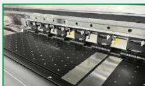
The printing platform is widened to ensure that the printing area is between the paper pressing slots to provide a stable printing effect
