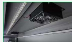
Standard fresh air system to reduce dust in the printing chamber and ink mist caused by inkjet.
