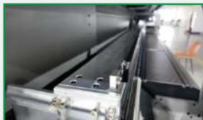
The aluminum profile main beam is used to replace the original steel structure, providing better mechanical strength and mechanical precision.
