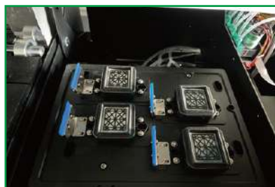
Automatic moisturizing function to extend the life of the heads
