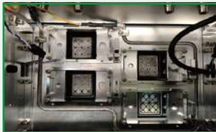
Adding bottom plate head heating to the car effectively improves printing stability
