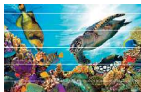
Gap / white streaks (Excessive paper feeding)
