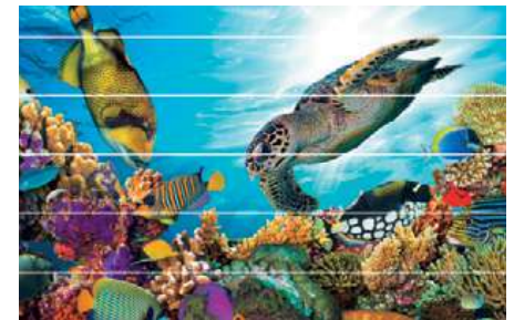
Gap / white streaks (Excessive paper feeding)
