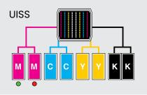
When the ink cartridge runs out of ink, the indicator will light up red, while the system already switches automatically to the second cartridge of the same color
